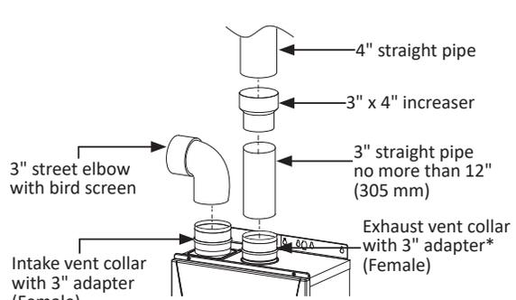
1. Insert no more than 12" (305 mm) of 3" straight pipe into the exhaust vent collar with 3" adapter.
