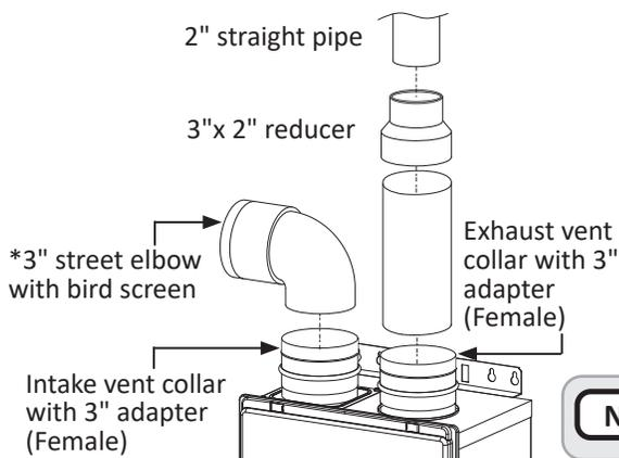
1. Insert no more than 12" (305 mm) of 3" straight pipe into the exhaust vent collar with 3" adapter.
