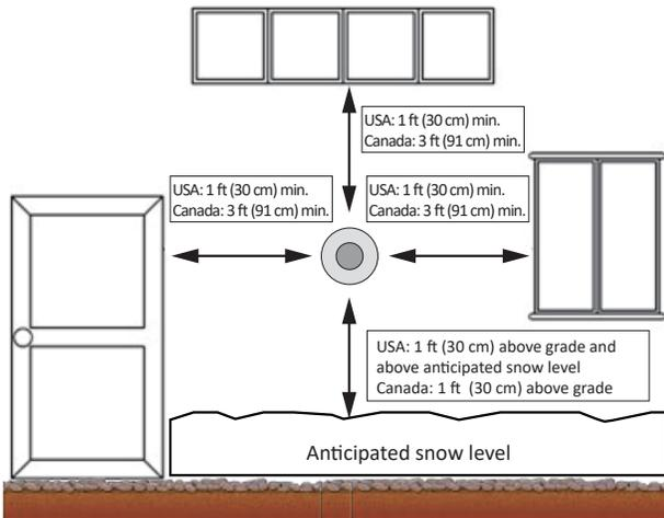
Ensure that you meet the minimum clearances shown below for Outdoor vent termination:
