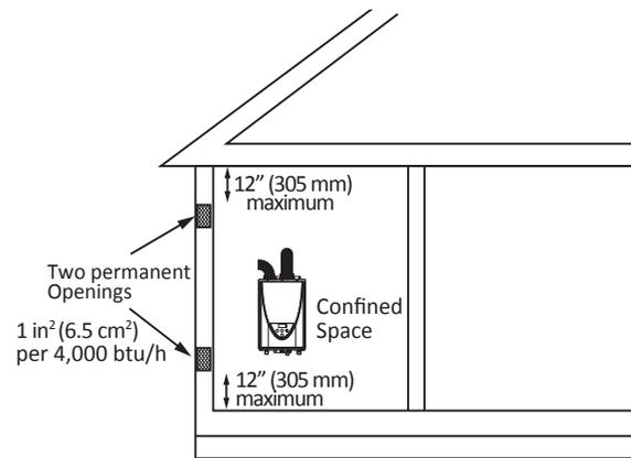
Figure 2 - Direct to outdoors openings
