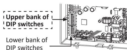
Set DIP switches shown in the table below depending on the vent diameter, the installation, and the vent length.
