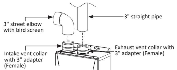
1. Connect spigot end of 3" street elbow into the intake vent collar with 3" adapter. Be sure to insert bird screen into the hub side.
