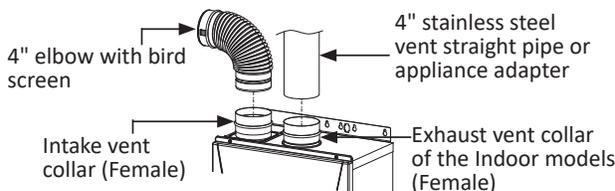
1. Connect a 4" stainless steel vent pipe or appliance adapter to the exhaust vent collar.
