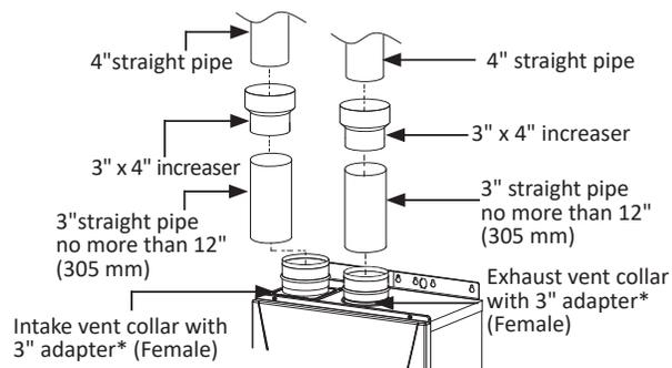
1. Insert no more than 12" (305 mm) of 3" straight pipe into the exhaust/intake vent collar with 3" adapter.
